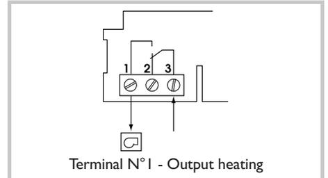
If your boiler is equipped with a thermostat input, remove the bypass of 2 thermostat terminals and connect them respectively to terminals 1 and 3 of the thermostat, to the 2 boiler's thermostat inputs (any connection scheme will do).
