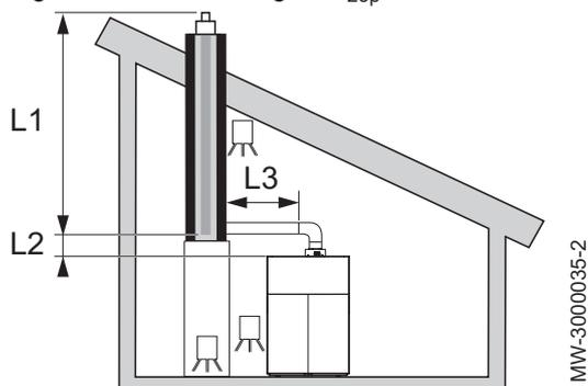
Fig.79 Fumisterie en traversée de toit B<sub>23p</sub>
