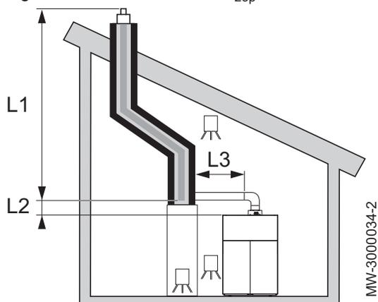
Fig.78 Fumisterie rigide B<sub>23p</sub>
